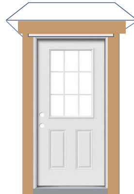
Install Window & Door Tape over Head Flashing
